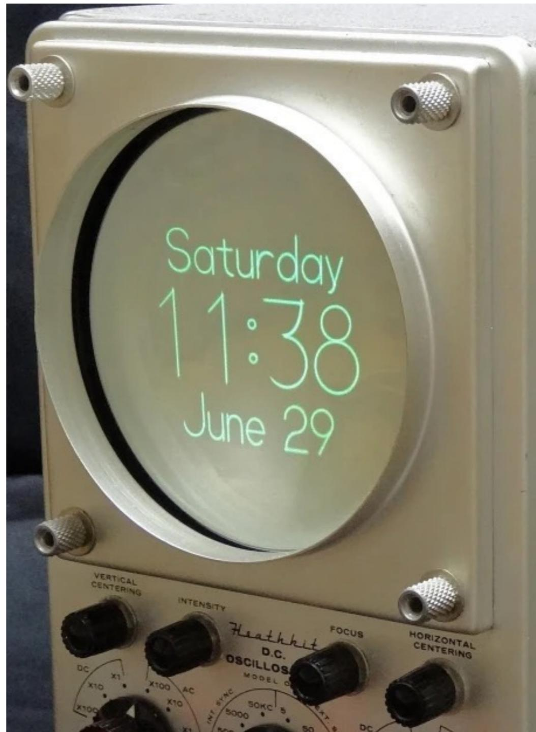
Oscilloscope Clock Using Hershey Fonts
